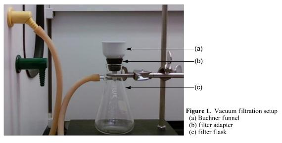
Check your filter flask for visible cracks or star cracks. If your flask is cracked, discard it and obtain a new flask from the stockroom. Attach one end of the thick-walled rubber hose to the
